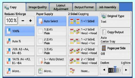
Select each tab and configure features as necessary; enter numbers of copy; press the <start> button to start a copy job.
