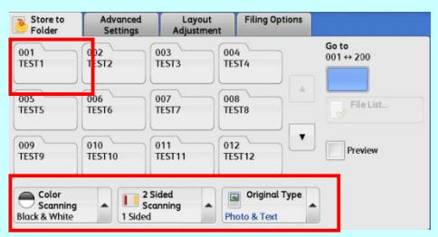
Select a folder to save the scanned data in; specify the features necessary; press the <start> button to scan & save the document in the folder.
